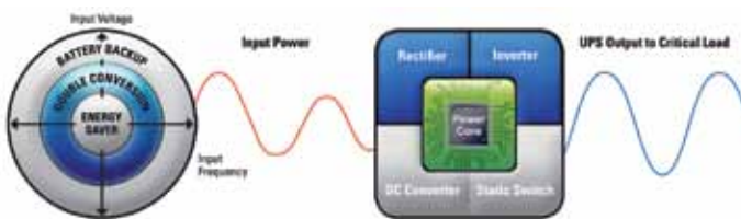
Input power quality within rectifier tolerance
